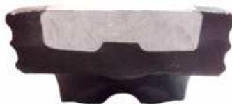
By bonding the elastomer to a phenolic backing ring, complete support and stability of the seat is assured. This guarantees positive control of seating torque while eliminating seat distortion.
