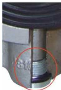
Plug used at the bottom of the valve, keeping lower stem not get out in any case, O ring on the plug offers third sealing to the stem.
